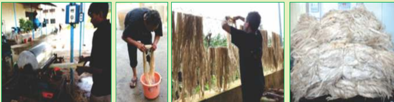
Fibre extraction, rinsing, drying and storing the dried fibres in bundles
