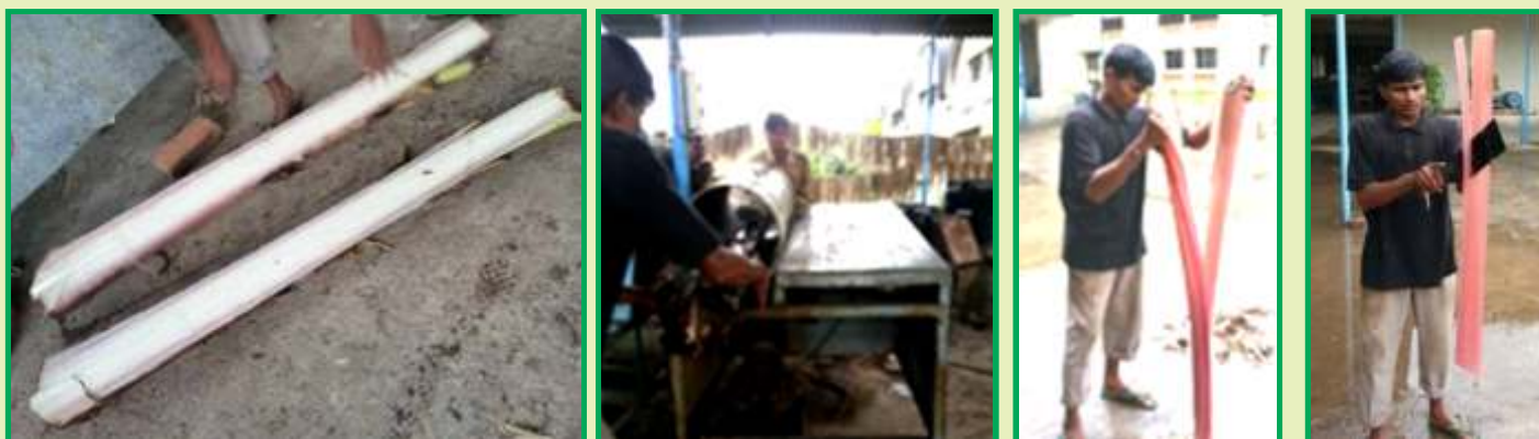
Splitting of pseudostem using cutter machine and separation of sheath
