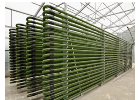
Tubular glass photobioreactor. Image: IGV Biotech, CC-BY 3.0
